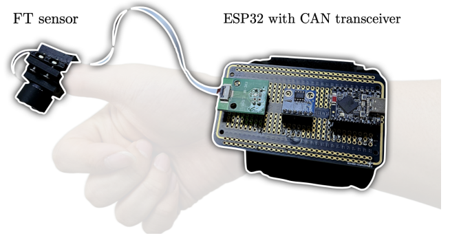
Fig. 2: Real force-data collection using a wearable F/T sensor. Contact interactions at multiple finger locations are synchronized with proprioceptive measurements.
